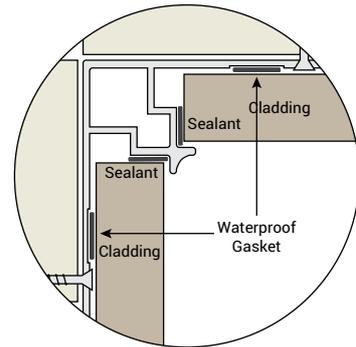
(12 x 10mm inner foam gaskets optional, alternative sealant option)
